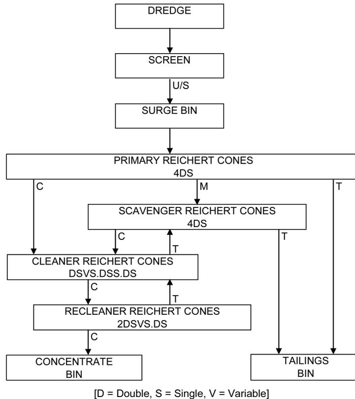
*Figure 1: Mining Pond B Cone Circuit*
