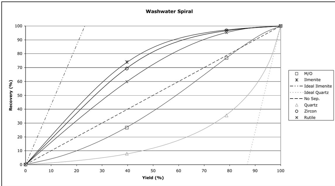
Figure 12: Summary of Test Data for the Wash Water Spiral
