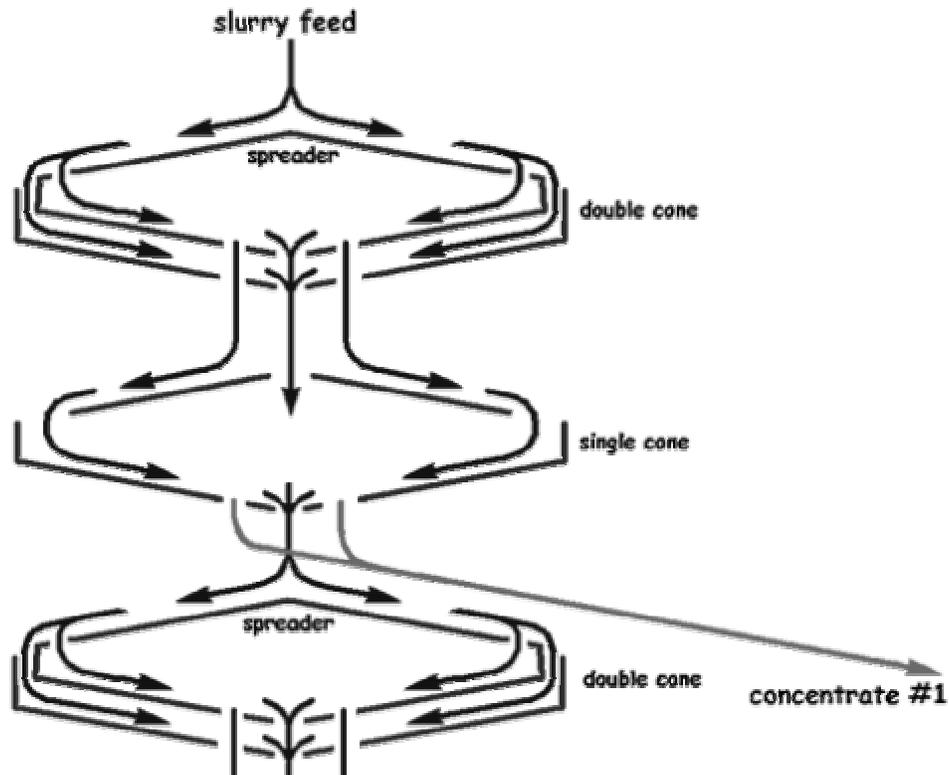
Figure 2: Reichert Cone Schematic showing the first three stages of a 4DS unit
