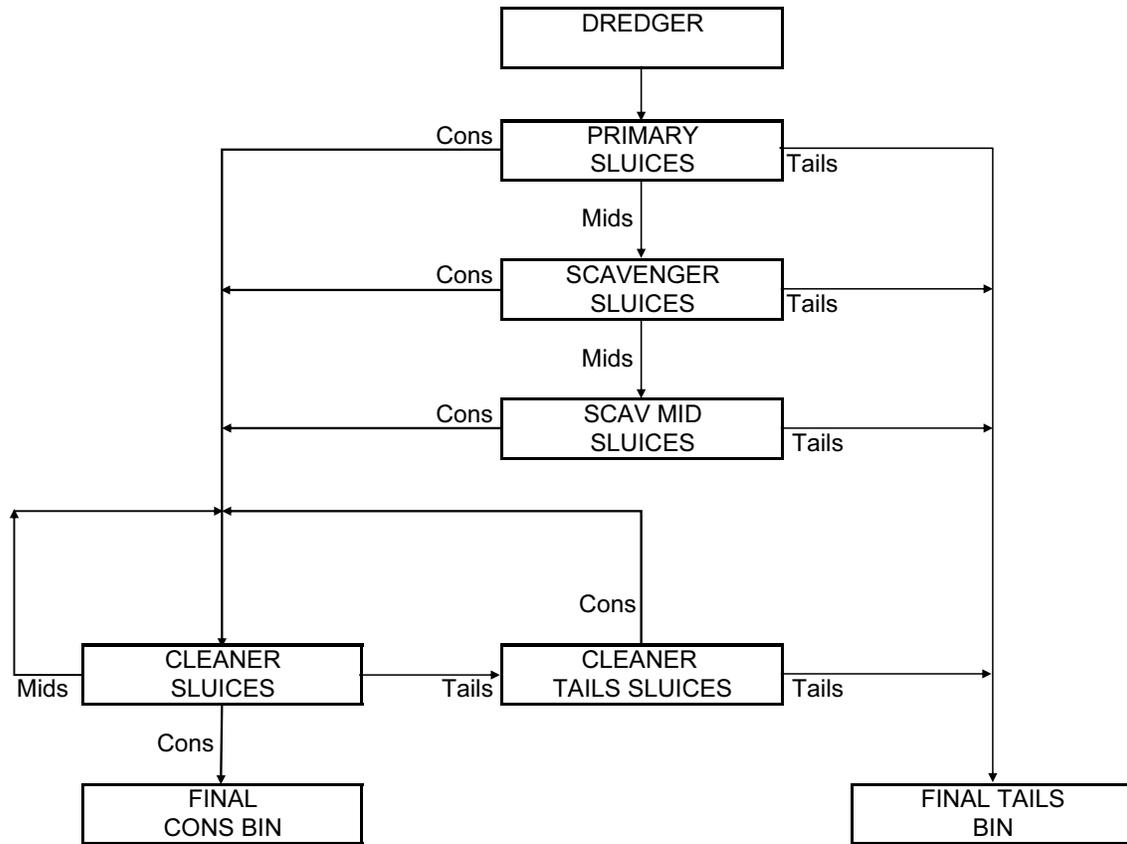
*Figure 3: A typical five-stage circuit*
