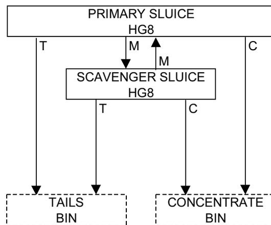
Figure 5: Current Feed Preparation Gravity Circuit
