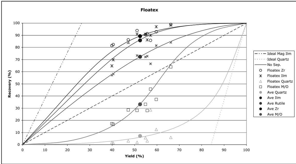
Figure 13: Summary of Test Data for the Floatex Hindered bed settler
