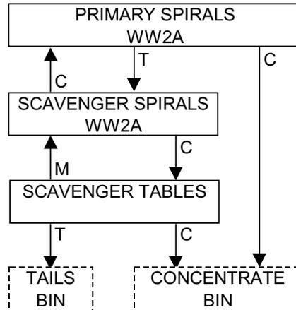
Figure 4: Original Feed Preparation Gravity Circuit Flow Sheet
