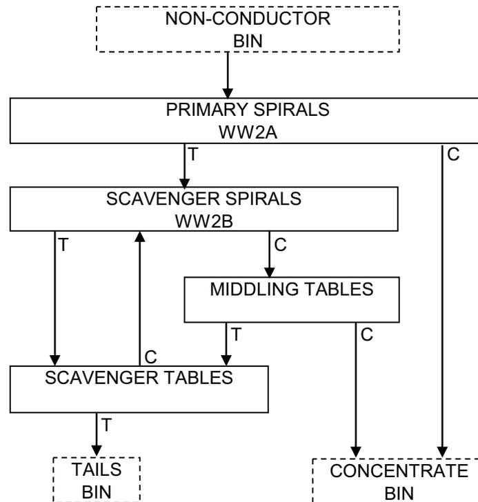
*Figure 6: Original Zircon Gravity Circuit*
