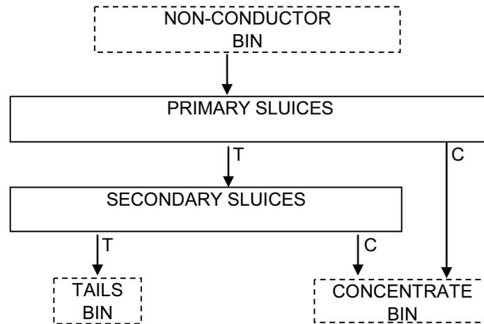
*Figure 7: Current Zircon Gravity Circuit*
