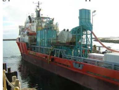
Figure 4 - Charter vessel based marine diamond sampling containerised plant (Courtesy BDM)
