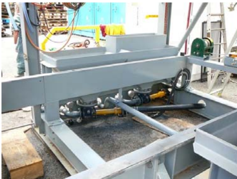
Figure 12 – Kelsey jig concentrate and tails jet pump hoppers
