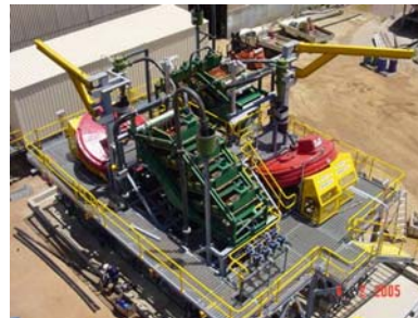
Figure 5 – Kelsey Centrifugal Jig Relocatable Plant for recovery of zircon from tailings dumps
