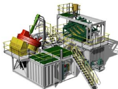
Figure 1 – Kelsey Centrifugal Jig Pilot Plant
