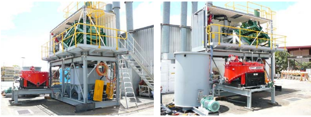
Figure 14 – KCJ unit maintenance slides – jig in maintenance position.
