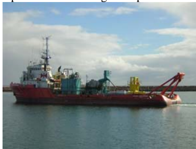
Figure 4 - Charter vessel based marine diamond sampling containerised plant (Courtesy BDM)
