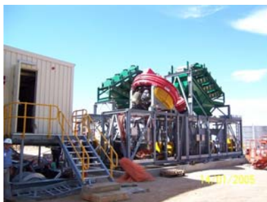
Figure 5 – Kelsey Centrifugal Jig Relocatable Plant for recovery of zircon from tailings dumps
